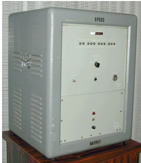
Figure 4.3: 1954 "DATRAC" 11-bit, 50-kSPS SAR ADC Designed by Bernard M. Gordon at EPSCO
