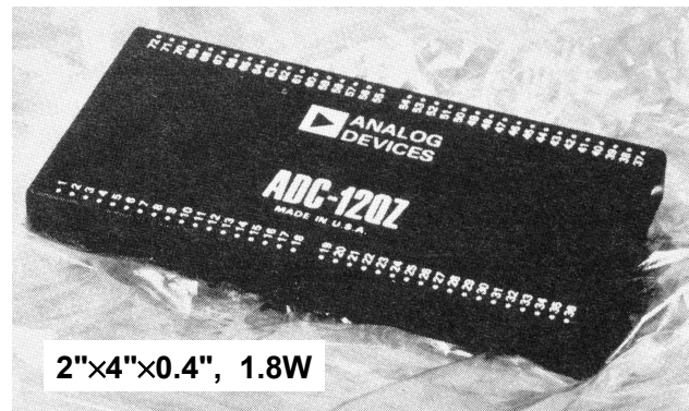
Figure 4.7: ADC-12QZ General Purpose 12-Bit, 40- \mu s SAR ADC Introduced in 1972
