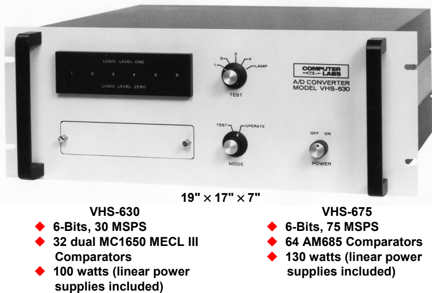
Figure 3.51: VHS-Series ADCs from Computer Labs, Inc. VHS-630 (1970), VHS-675 (1975)
